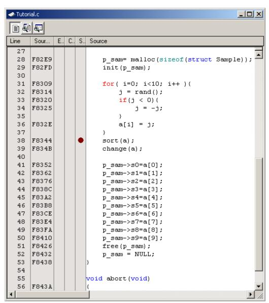
Figure 3.4 Editor window (setting a software breakpoint)
